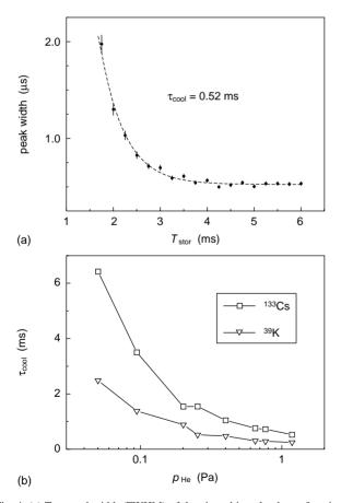
Fig. 4. (a) Temporal width (FWHM) of the ejected ion cloud as a function of the storage time  $T_{\rm stor}$  in the linear RFQ ion trap, measured on an MCP detector about 1 m downstream [29]; (b) dependence of the cooling time constant  $\tau_{\rm cool}$  on ion mass and buffer gas pressure [29]. The solid lines are meant to guide the eye.
