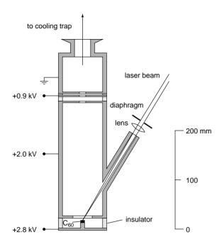
Fig. 6. Detailed sketch of ISOLTRAP's carbon cluster ion source, which is mounted about 2.5 m upstream of the cooling Penning trap [33]. The carbon cluster ions are obtained from laser desorption, fragmentation, and photo-ionization of a  $C_{60}$  pellet and are electrostatically accelerated towards the cooling Penning trap.
