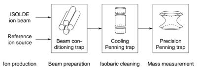
Fig. 1. Sketch of the main components of the ISOLTRAP mass spectrometer and their functions.
