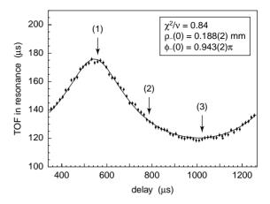
Fig. 10. Time-of-flight in resonance, i.e., at the centroid minimum, as a function of the delay between the start of the measurement cycle and that of the magnetron excitation, corresponding to a phase difference of 0 to  $2\pi$  [36]. The delays marked by arrows correspond to the phase differences (1)  $\Delta\phi_- = 3\pi/2$ , (2)  $\Delta\phi_- \approx 0$ , and (3)  $\Delta\phi_- = \pi/2$ . The solid line is a fit of the theoretical curve to the data points.
