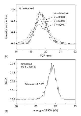
Fig. 5. (a) Simulated temporal distribution of an ion pulse extracted from the RFQ ion beam cooler and buncher and accelerated to 30 keV for different initial temperatures (lines) and measured distribution (squares) [29]; (b) calculated energy spectrum of an ion pulse corresponding to the 300-K pulse shape of (a) [29]. All simulations and measurements were performed with <sup>133</sup>Cs.
