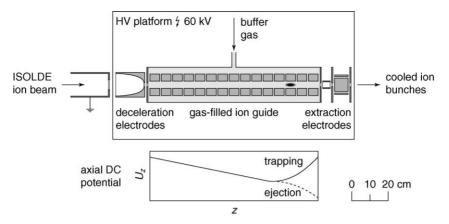
Fig. 3. Sketch of the radiofrequency ion beam cooler and buncher. See the detailed description in the text.
