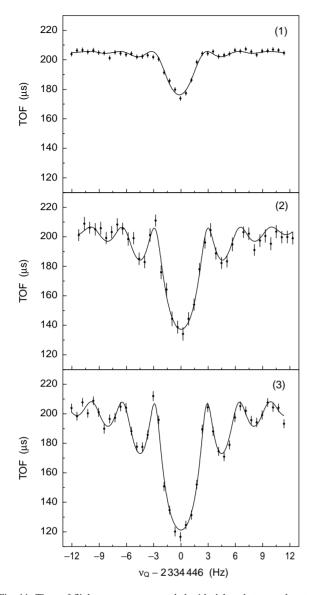
Fig. 11. Time-of-flight resonances recorded with delays between the start of the measurement cycle and that of the magnetron excitation corresponding to the three phases marked by arrows in Fig. 10 [36]. The solid line are fits of the theoretical function [17] to the data points.
