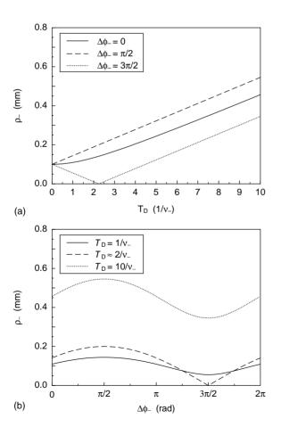
Fig. 9. (a) Calculated final magnetron radius as a function of the duration of the dipolar excitation for three values of the phase difference between the excitation and the initial magnetron motion [36]; (b) calculated final magnetron radius as a function of the phase difference between the excitation and the initial magnetron motion for three different excitation durations [36].
