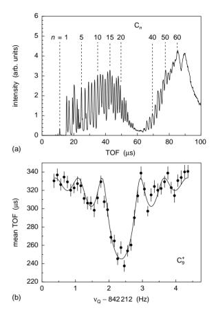
Fig. 7. (a) Time-of-flight mass spectrum of carbon cluster ions produced with ISOLTRAP's carbon cluster ion source, recorded on an MCP detector mounted about 1 m above the source [34]; (b) time-of-flight resonance of  $C_9^+$  [18]. The solid line is a fit of the expected line shape [17] to the data points.
