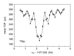
Fig. 2. Time-of-flight resonance curve of  $^{85}$ Rb<sup>+</sup> at an excitation time of  $T_{\rm Q}=1.8\,{\rm s}$ . The solid line is a fit of the theoretically expected line shape [17] to the data points.
