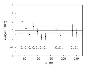
Fig. 8. Deviations of the weighted means of the measured carbon cluster ion masses from their true values after correction for the mass-dependent systematic effect [18]. The dashed lines indicate the residual systematic uncertainty.
